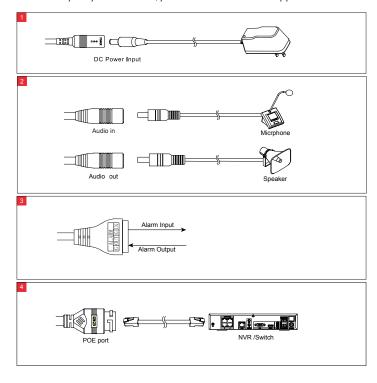
NOTE: All external devices should be powered separately. There is no power voltage from the camera.
