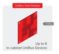
UniBus Devices are designed for installation within the same enclosure as the UniBus host module. A UniBus host can interface a maximum of six UniBus devices in any combination, provided they are all within the intended functionality of the host module
