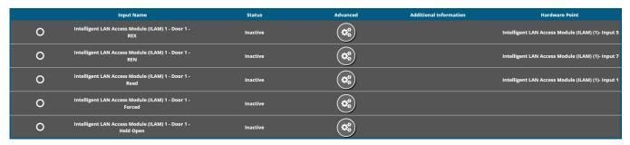
Similar to the traditional hardwired door's *Door Side Settings*, the only difference for Aperio locks is that the *Outside Reader* and *Inside Reader* cannot be set. This is due to the Inception system automatically assigning the Aperio lock's only reader as the *Outside Reader*.
