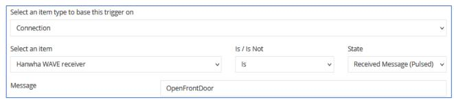
NOTE: If the message text sent from wave includes spaces Inception will receive them as x20 and the trigger must reflect this. i.e.
