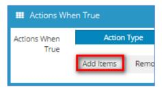
This example will allow Wisenet WAVE to open a door. Select Control Door, Front Door and Grant Access. Click on *Confirm*.
