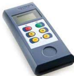
Figure 2: Salto PPD used to program the Salto Router and Salto Locks
