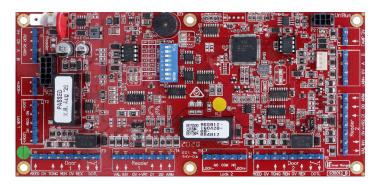
In normal operation, the ILAM connects to an Inner Range Controller via the RS-485 LAN or IP LAN if using an Ethernet Bridge or CLOE module. When a credential is presented to an ILAM's reader, the ILAM sends a message to the Controller to notify it of the access attempt. The Controller determines if access should be granted and responds to the ILAM. The ILAM then provides feedback via its outputs, the reader LEDs & beeper, and activates lock relays if access is granted.
