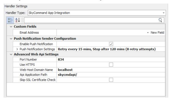
The Skycommand App Communication Handler is configured with an email address, used to connect Skycommand accounts to a User in Integriti, determining the permissions that account will have for viewing/controlling Entities in Integriti. Push Notifications are enabled by default and their retry period and attempts can be configured, defaulting to every 15 minutes, retrying 8 times.
